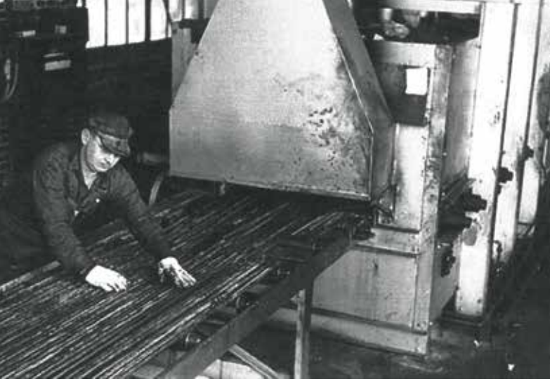
True Temper "Tube Mill" in Geneva, Ohio. Once the tubes are drawn to size they are pushed through a series of reducing dies.
