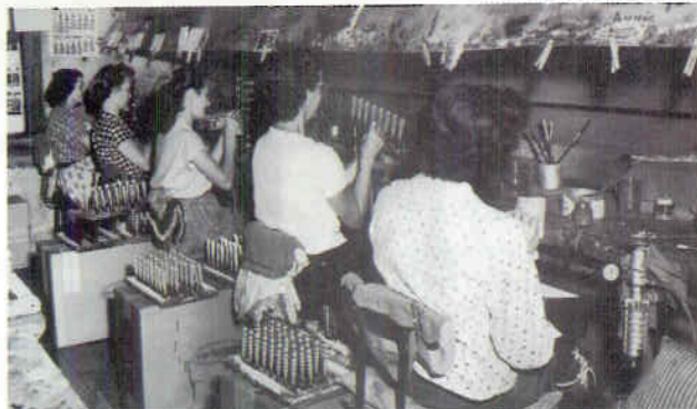
With air brushes and steady hands, employees of the paint finish department add the final touch to the lures.
