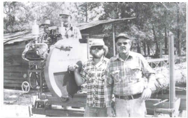
This 1981 photo, taken by Mr. Carter's wife Essie, features Mr. Carter at the controls of his new Oregon Mills Mobile Dimension Saw, which he purchased with the assistance of Mr. William Cleckley (center). The saw mill allowed for the numerous stands of mature cypress, aged from 250 to 375 years old (according to core samples taken by NFWFMD biologists) to be cut on site for the many bridges, dikes, dams and retention walls needed on the property. Mr. Cleckley's father, James Robert Cleckley, is pictured on the right. The Cleckleys were neighbors of Mr. Carter, and William, now Director of the Division of Land Management and Acquisition, Northwest Florida Water Management District (NFWFMD), still owns property adjacent to the Fitzhugh Carter Tract. Photo courtesy of Mr. Bill Cleckley, NFWFMD.
