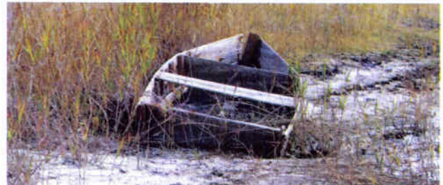
Above: Two of Mr. Carter's many boats made of cypress cut from the Chain Lakes swamps. They still occupy their last mooring, mired in the mud along a lake shore. Note the heavy application of tar used with caulking material to seal up the seams in the boards.
